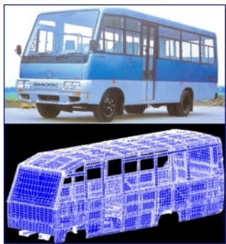
Full Vehicle Simulation using SolidWorks Simulation
