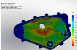
Gearbox cover stiffness improved using material only where it is required
