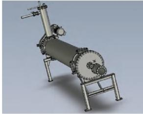
Bouldin & Lawson's patented steam chamber or Hydrolyser, one-of-its-kind design, to continuously transform the processed waste into a safe and multi-use by-product. The steam chamber makes the transformation much faster, more economical, and more environmentally friendly than other waste conversion technologies. (Diagrams courtesy of Bouldin Corp.)
