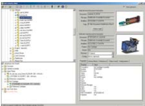
To facilitate collaboration, some PDM software systems allow non-CAD users such as manufacturing and purchasing staff to access all documents and to add non-CAD documents to the vault.
